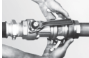
2. Cam arms lock coupler and adaptor together.
