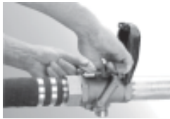
2. Press push button and lift locking arm.
