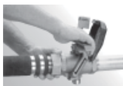
3. Bring the disc faces together and slide downward.
