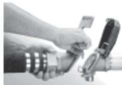
3. Remove the coupler from the adapter.
